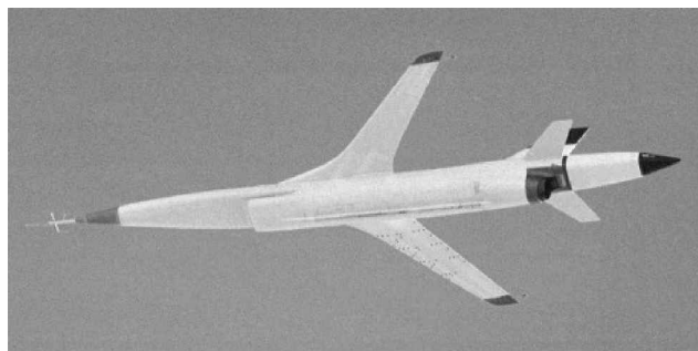
Fig. 9 Drone for aeroelastic and structural testing in flight, 1984.
